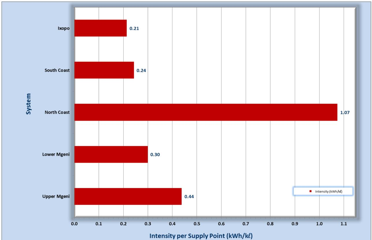
Figure 4.2 Energy requirement to treat water in Umgeni Water Systems 2015/16.
