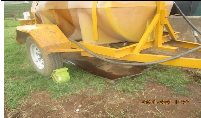
Figure 1: Damaged drip tray placed under petrol tanker
